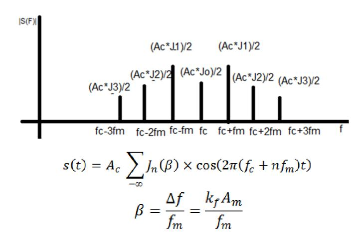
The spacing between spectral lines equals fm You should observe this spectrum in the experiment
